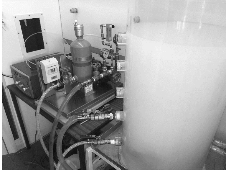
Figure 5 – 1. Microbubble generation experimental apparatus.
