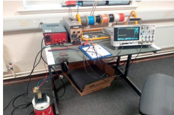
Figure 4. Experimental setup to monitor intermittence using oscilloscope
