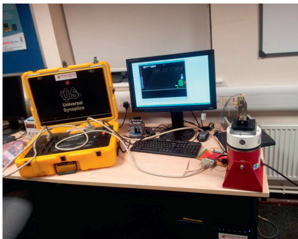
Figure 3. Experimental setup to monitor intermittence using n-compass
