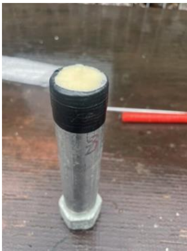
Figure 5: Left image: Pipe bomb rigged for high order detonation with PENO donor charge visible.
