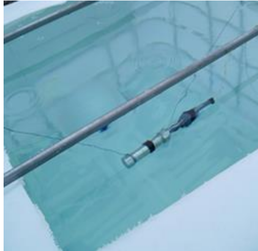
Figure 4: Pipe bomb suspended in 1000l IBC tank for low order deflagration.
