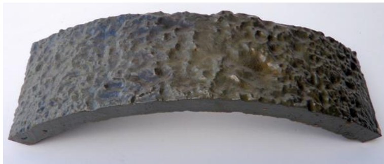
Figure 3-4: Characteristic pitting in water mains pipe due to soil-water corrosion (Picture: S. Hallett)
