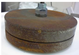
Figure 3: Surface corrosion of metal discs
