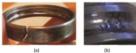
Figure 4: Bearing with fracture (a) outer ring failure and (b) inner ring failure (Source: (Medjaher et al., 2012))
