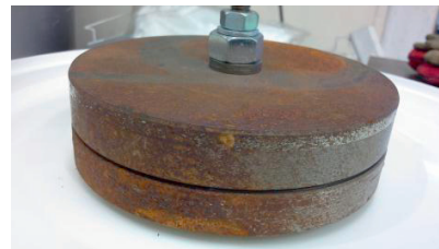
Fig. 1: Metal discs showing corrosion on the surface
