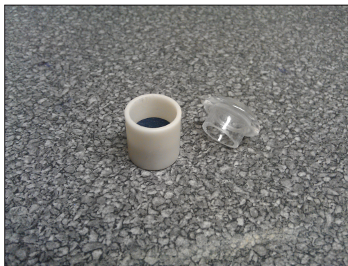
(b) A single bulk sample pellet inside an alumina crucible with silica lid
