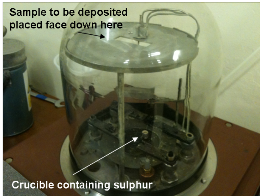
Figure 3.5: Image of the thermal evaporation equipment used to sulphurise metallic precursors
