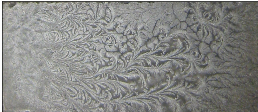
(c) Sample 3 - a double anneal of 30 min at 250 °C then 30 min at 500 °C produced a swirly pattern of opaque grey film with many gaps between the swirls
