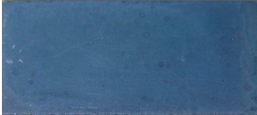
(a) Sample 1 - a single anneal of 30 min at 250 °C produced a solid dark blue film
