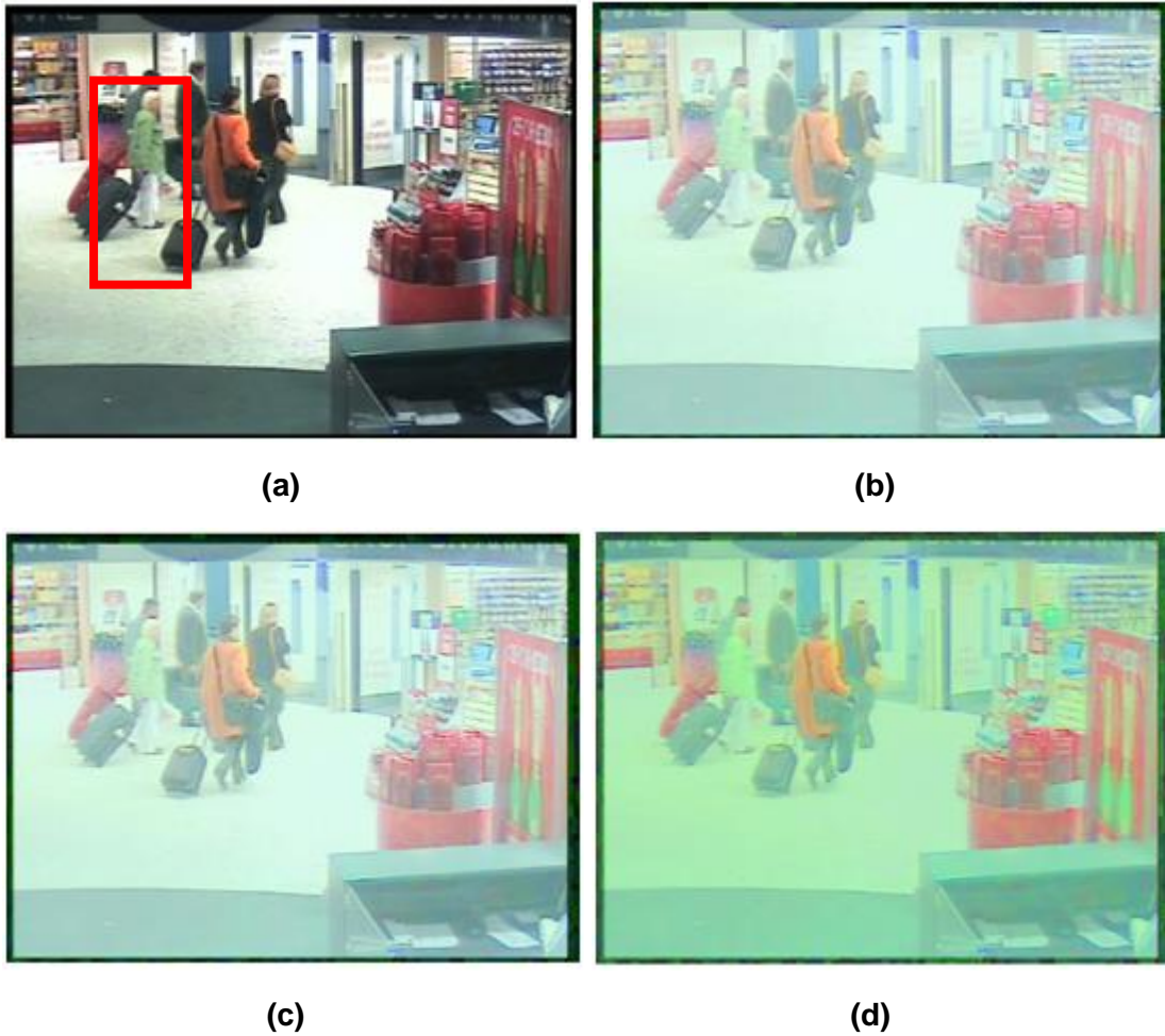
Figure 4-7: Shows MSR-CR result. (a) Raw/original Image with Target (red box) in cam 1. (b) MSR-CR result with surround constants c_1=15 , c_2=80 , c_3=250 , gain G=192 , offset b=-30 , \alpha=125 and \beta=46 (c) MSR-CR result with surround constants c_1=15 , c_2=80 , c_3=250 , gain G=50 , offset b=-3 , \alpha=125 and \beta=46 (d) MSR-CR result with surround constants c_1=15 , c_2=80 , c_3=250 , gain G=192 , offset b=-30 , \alpha=10 and \beta=5
