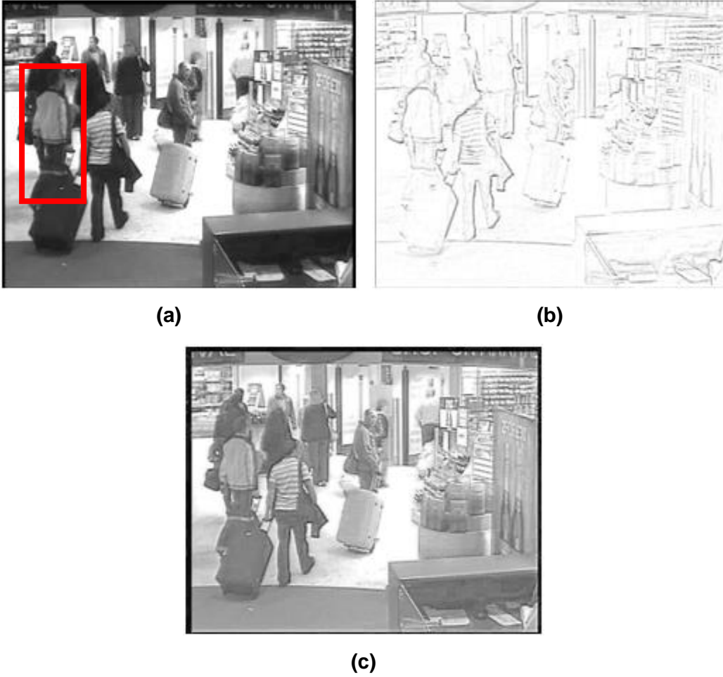
Figure 4-4: Outlines the ‘reflectance’ and one-band intensity map: (a) the intensity I(x,y) of original image for Target (red box) in Cam1 (b) luminance based ‘reflectance’ image obtained by equation (4.3) (c) the one-band enhanced intensity I_{enh} by using equation (4.14).
