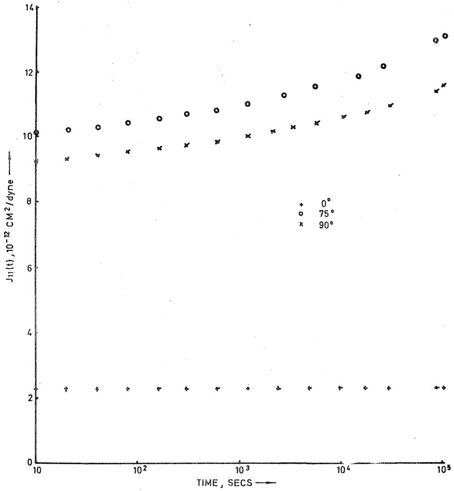
FIGURE 4 VARIATION OF CREEP COMPLIANCE WITH TIME.  $V_f = -48, X = -39, Y = 61.$
