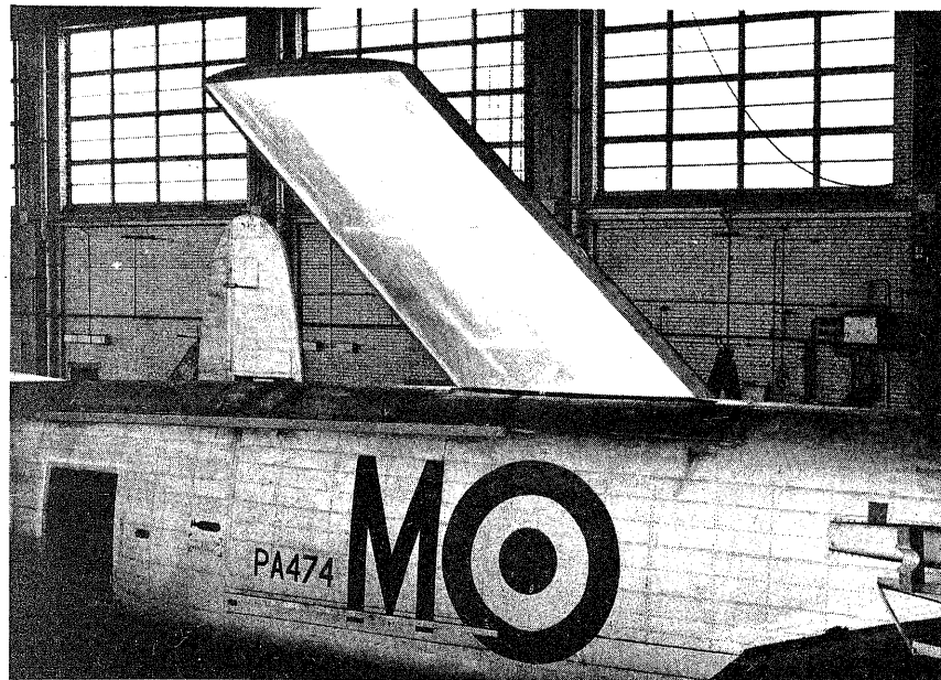
FIG. 5. SWEEP BACK HALF WING IN POSITION.
