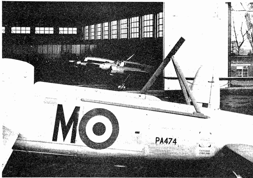
FIG. 2 PRESSURE PLOTTING MAST IN AFT POSITION.
