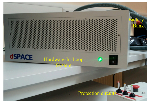
Fig. 4b dSPACE™ HIL system
