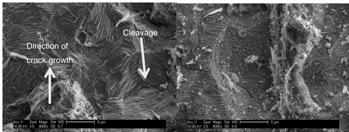
Figure 6-44 Ductile striations on parent materials in seawater \Delta K=19\text{MPa}\sqrt{m}
