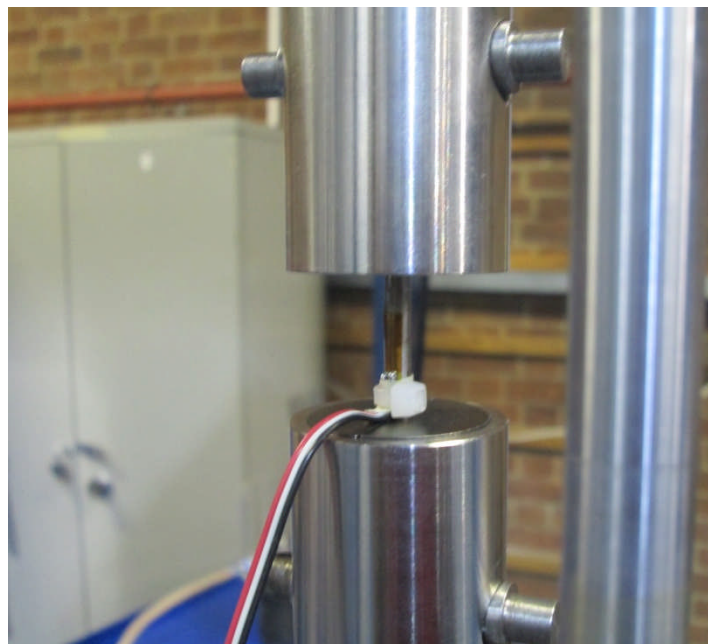
Figure 3-3 Load and alignment check
