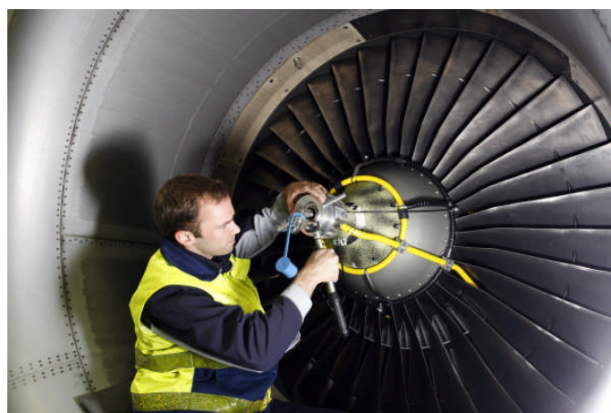
Figure 2.23. Cycleclean ™ Engine Wash System developed by Lufthansa Technik [35]
