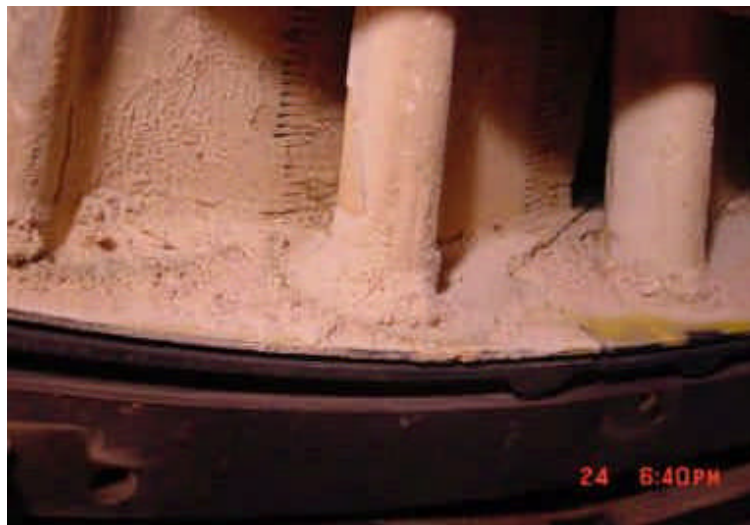
Figure 2.4. Gas turbine fouling [Basendwah, 2004]
