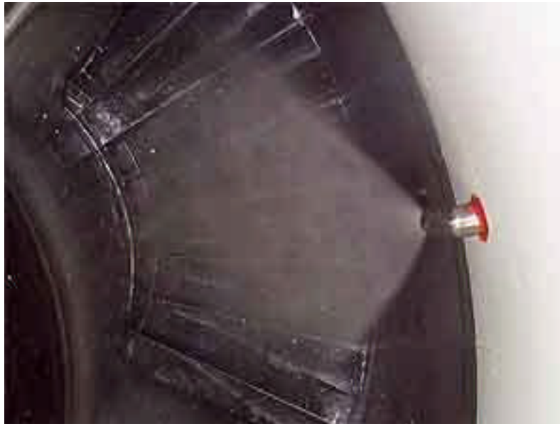
Figure 2.11. Offline cleaning injection pipe [Margolis, 1991]
