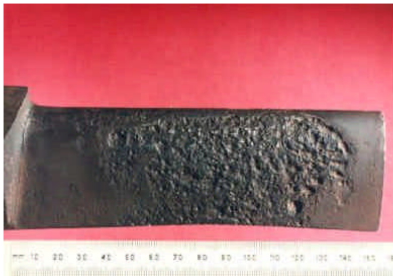
Figure 2.6. Compressor blade corrosion [Grewal, 1988]
