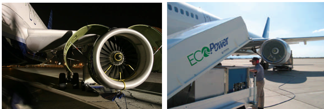
Figure 2.22. P&W's EcoPower ® compressor washing system [51]
