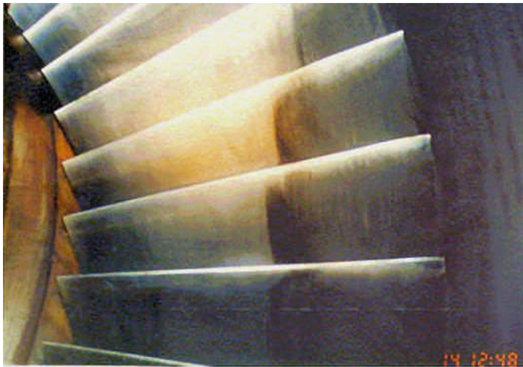
Figure 2.3. Industrial gas turbine compressor fouling [Basheer, 2006]
