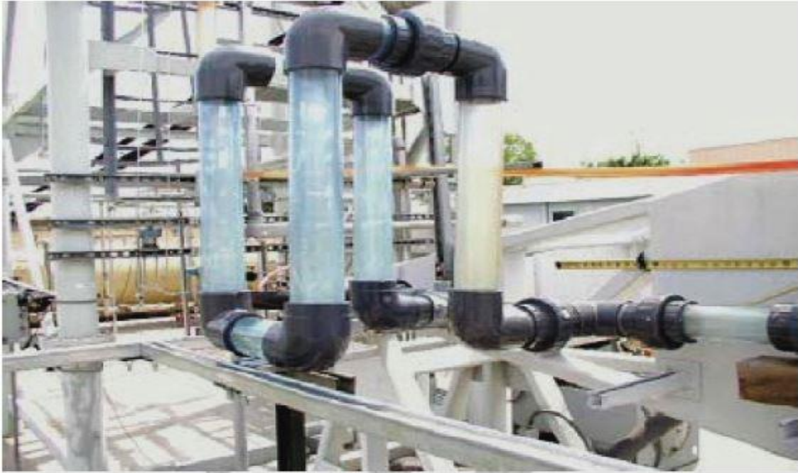
Figure 2-15 Non- intrusive passive slug attenuation device [107]
