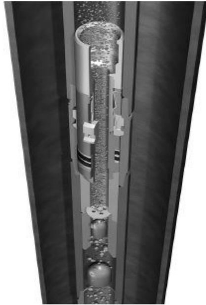
Figure 2-14 Diagrammatic representation of Bubble Breaker [114]
