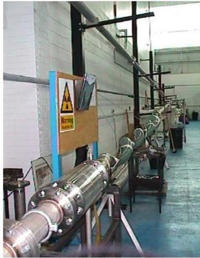
Figure 2-11 Novel pipe device for severe slugging attenuation [109]
