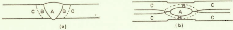
FIG.1 REGIONS IN A BUT WELDED JOINT
