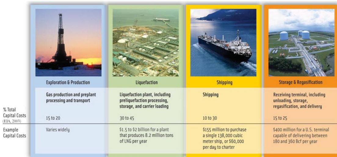
Figure 6: Showing the four main steps of the LNG value chain (NETL, 2005)
