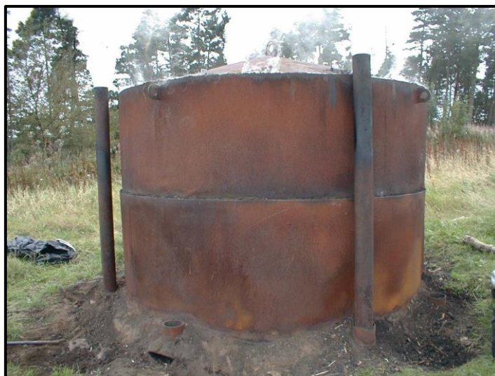
Figure 2-1: Tropical Products Institute metal ring kiln used to produce biochar. (Photo courtesy of David Hutchinson, received 2009)
