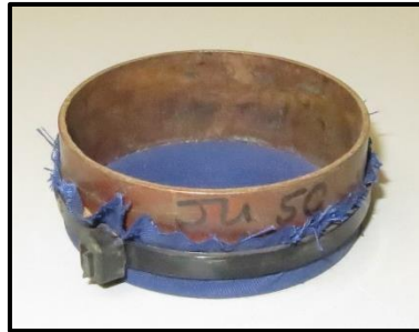
Figure 3-2: Metal ring used for the water release curve. Mesh base secured in place with cable-tie which would not degrade during the experiment.
