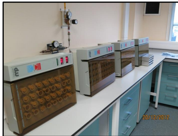
Figure 4-5: Measurement of carbon dioxide release in progress with the Rapid Automated Bacterial Impedance Technique (RABIT). Each unit contains 32 locations for the sealed containment tubes.
