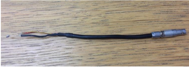
Figure 52 LEMO FGG.00 temperature measuring connector and sensor
