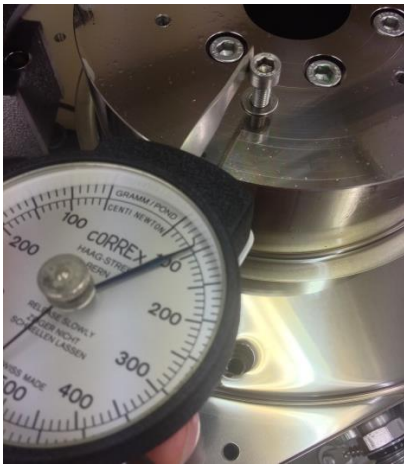
Figure 78 The start rotating force of the bearing spindle under uneven journal bearing pocket pressures
