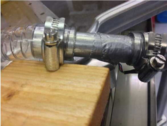
Figure 55 Temperature sensor Tai1 and Tai2 to measure the oil flowing out from the pump
