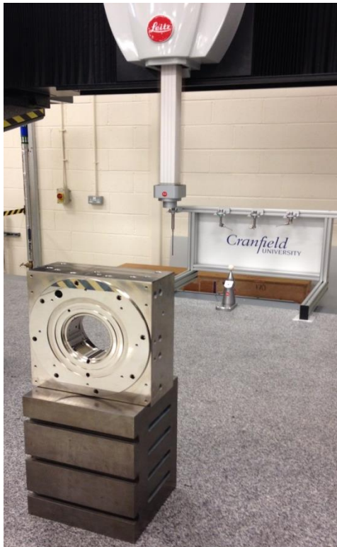
Figure 39 The bearing house is being measured by the Leitz CMM
