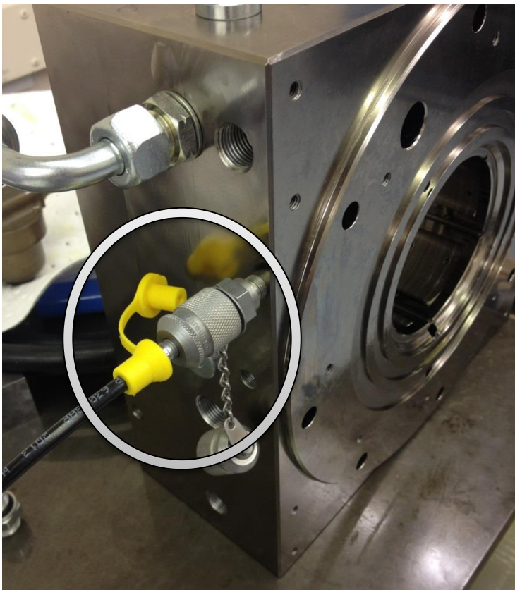
Figure 48 Hole on the bearing housing to insert the pressure gauge
