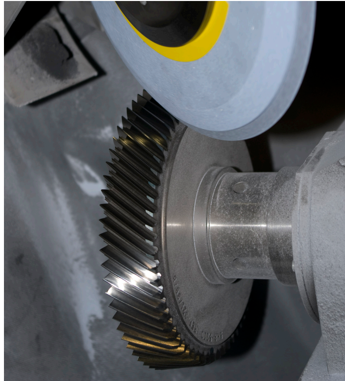
Figure 7.1: Generation of a helical cutter with a grinding wheel. The wheel shape corresponds to the former, which represents a corrected rack tooth profile [148].
