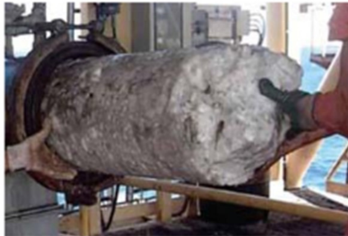
Figure 15 Hydrate formation flow challenge in ultra-deepwaters
