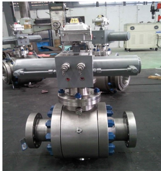
Figure 28 Subsea hydraulic ball valve, courtesy of Weiku.
