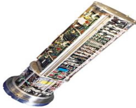
Figure 40 Subsea Electronic Module (SEM), courtesy of Weatherford
