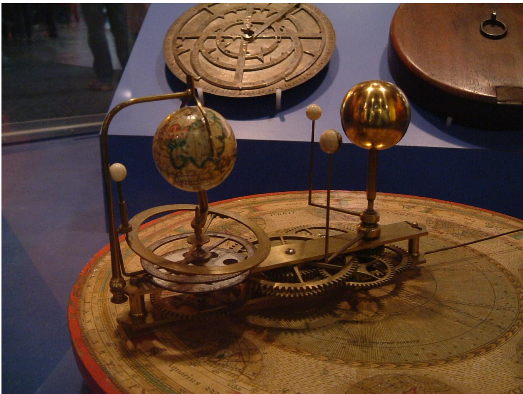
Figure 2 - A relatively simple orrery modelling Mercury, Venus, Earth and the Moon (image credit: Kaptain Kobold, 2006, Flickr via Wikipedia)
