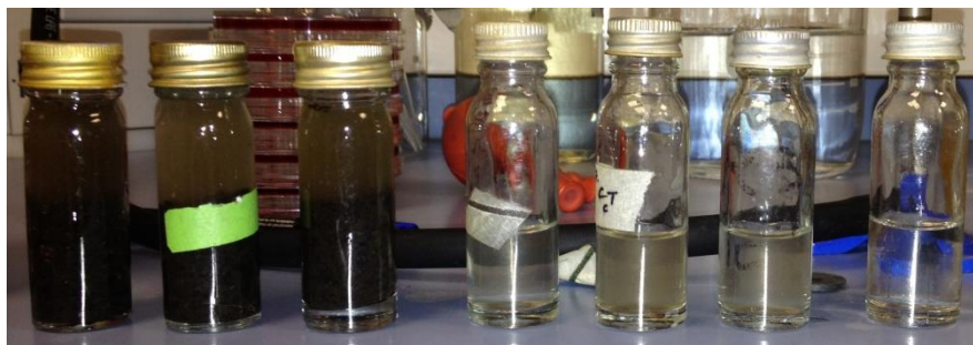
Figure 2.4 – The three bottles to the left show the 5g samples of sludge cake in a universal bottles following the addition of 10 ml MRD prior to vortexing. The four bottles to the right are preparation for serial dilution.
