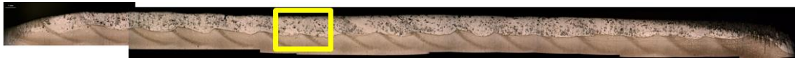
Figure 9-17: microsection of GTA cladding trial on 460 mm outer diameter railway brake disc; yellow window: extract shown in figure 9-18; left: inner diameter, start cladding; right: outer diameter, finish cladding
