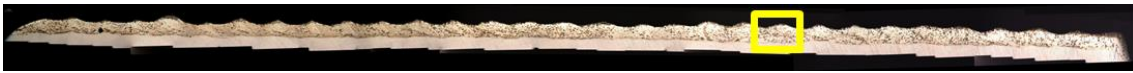
Figure 9-8: Microsection of GTA cladding trial on 640 mm outer diameter railway brake disc; yellow window: extract shown in figure 9-9; left: inner diameter, start cladding; right: outer diameter, finish cladding
