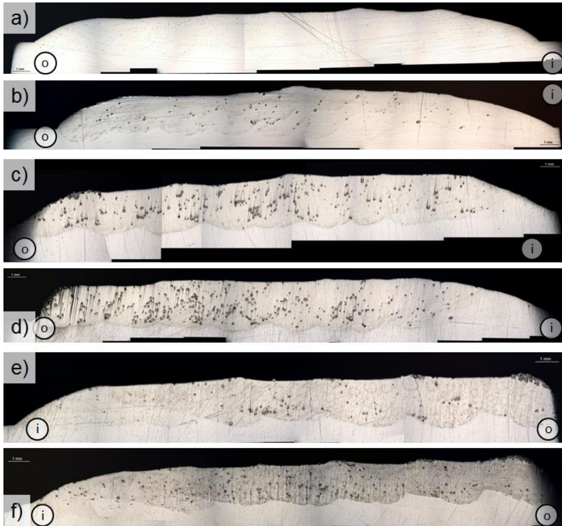
Figure 8-7: Control microsections of specimen welds like those of the POD wear test specimen; a) PFR = 0 g/min; b) PFR = 5 g/min; c) PFR = 10 g/min; d) PFR = 15 g/min; e) PFR = 20 g/min, cracks have been found; f) PFR = 25 g/min, cracks have been found; i: inner side of the spiral, o: outer side of the spiral
