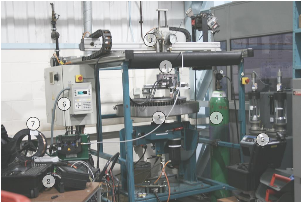
Figure 9-1: GTA brake disc cladding with WC powder, overview of the welding rig; 1: TIG torch on z-axis; 2: Turntable with brake disc mounted on; 3: Pressure releasing container with valve; 4: Ar transport gas bottle; 5: Powder feeder; 6: 5-axis-rig controller; 7: KT4 wire feeder; 8: AMV display and recorder (arc current, arc voltage and wire feed speed)
