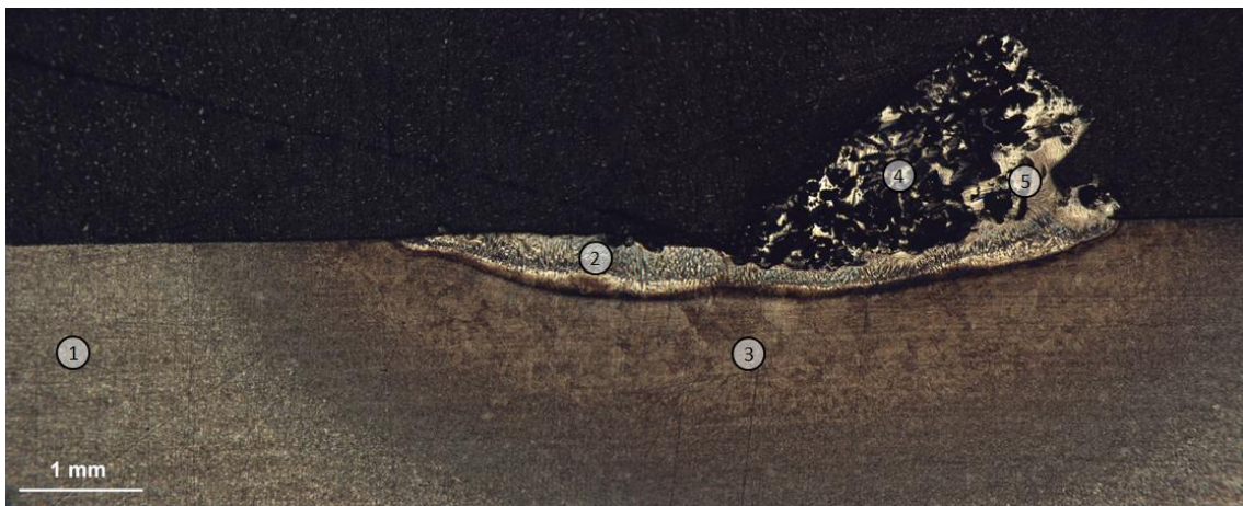
Figure 11-1: autogenous PTA cladding trial with SiC feeding on steel; 1: steel base plate; 2: weld area; 3: HAZ; 4: bonded SiC particles; 5: steel and SiC mixed
