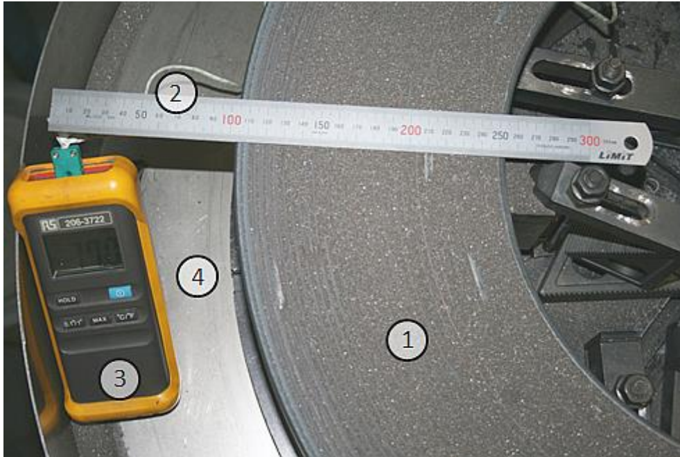
Figure 9-5: Typical temperature measurement of the brake disc during welding; Temperature display; 1: brake disc; 2: thermocouple lead; 3: temperature display apparatus; 4: powder tray
