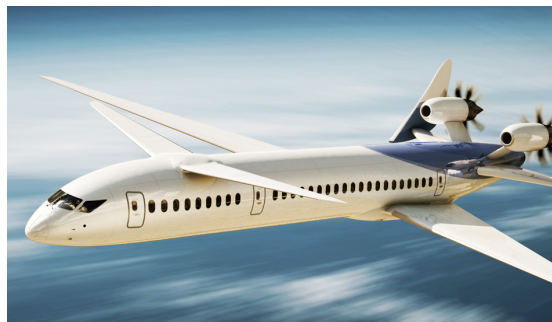
FIGURE 6.25: Possible future civil airliner with rear-mounted engines and canards [3]
