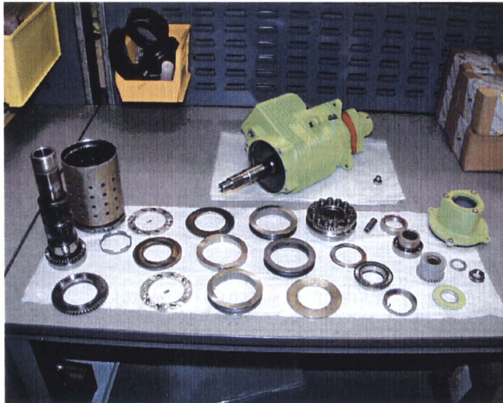
Figure 2.3-2 – Components Removed from the Skewed Roller Device.
