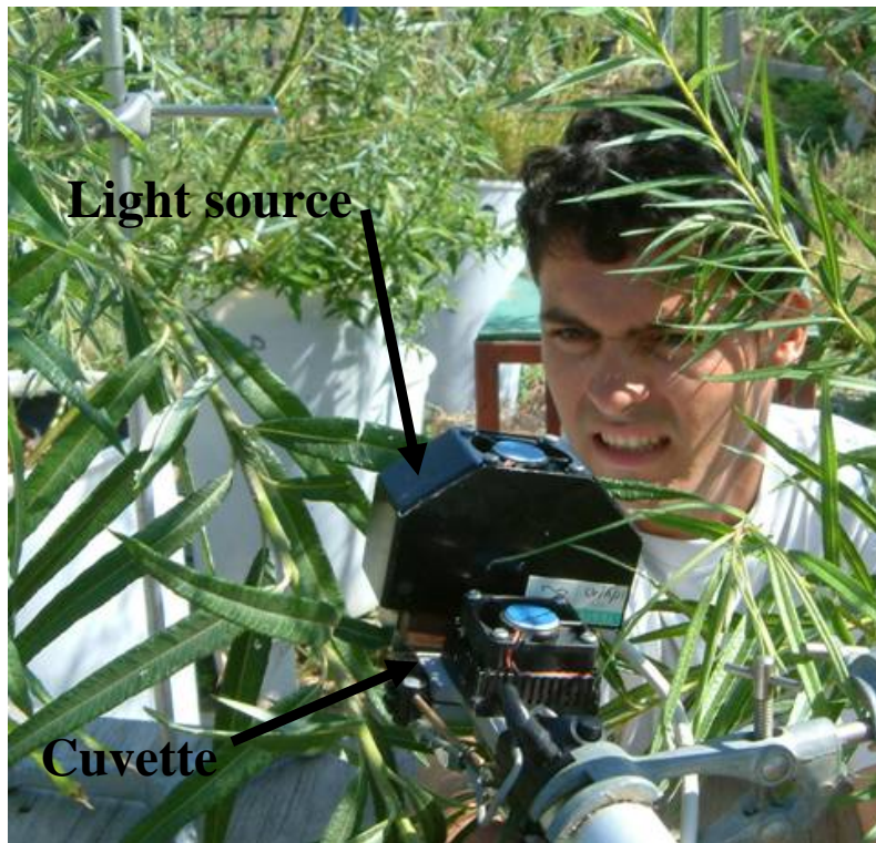
Plate 9. Using the CIRAS-1 on willow leaves, Lysimeter trial; Silsoe; Bedfordshire; 2003.
