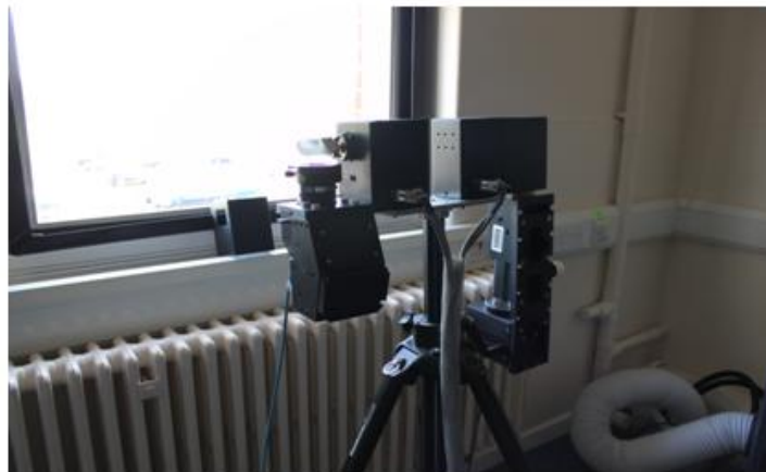
Figure 3 The Headwall Visible Near Infra-red (VNIR) imaging system.
