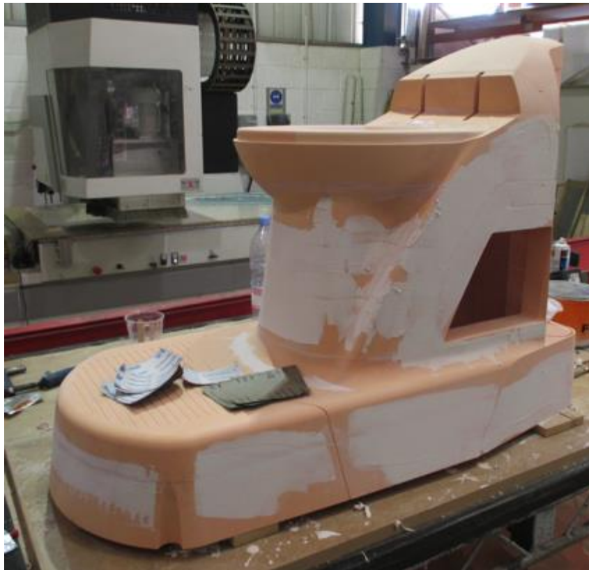
Figure 74 - Dense modelling foam having been machined now being assembled (C4D, Cranfield University. Ross Tierney © 2014)
