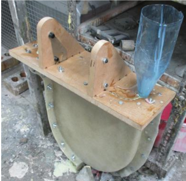
Figure 76 - Toilet lid being cast in blue resin (C4D, Cranfield University. Ross Tierney © 2014)
