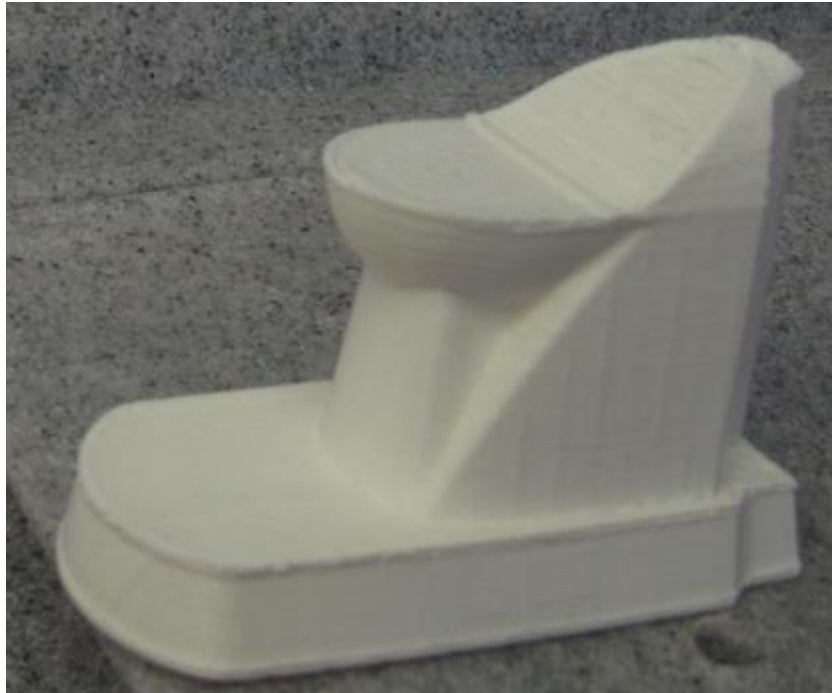
Figure 57 - 3D Print of Full Toilet to scale of 1:10 created during the latter development stage of Case Study (C4D, Cranfield University. Ross Tierney © 2014)
