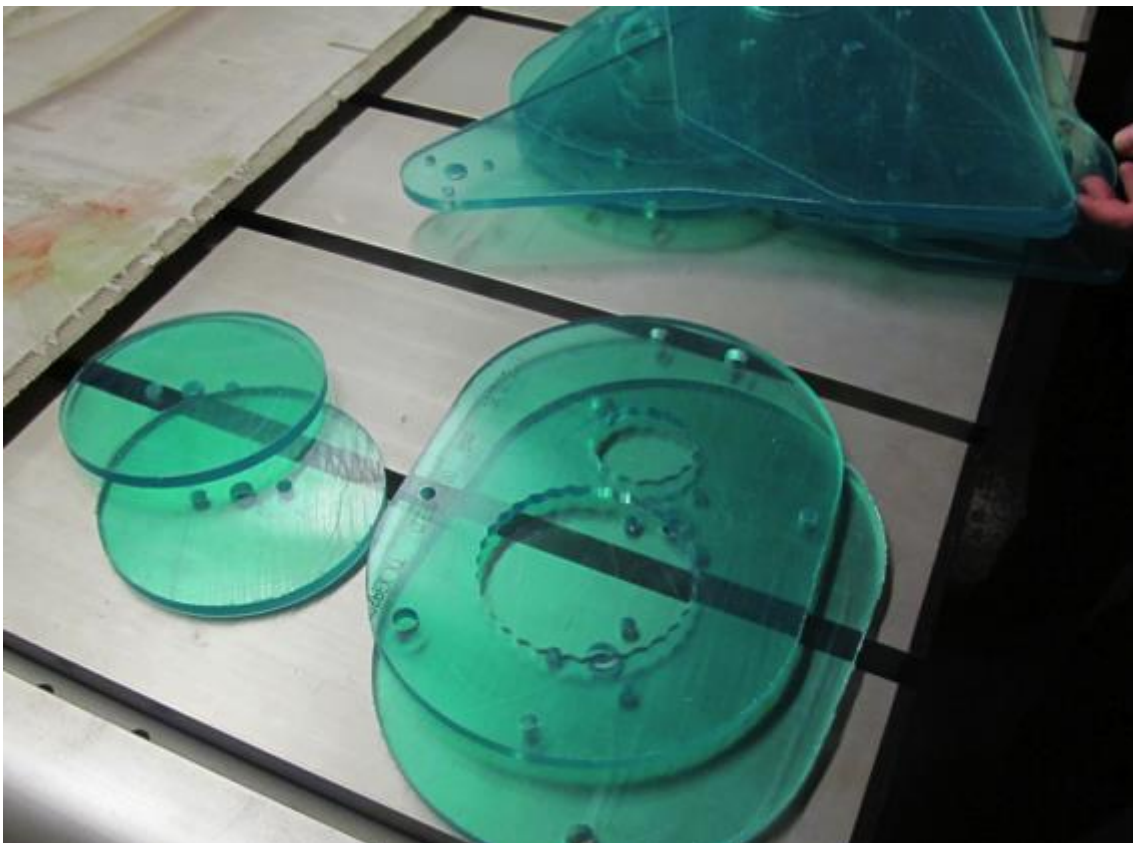
Figure 45 - Pieces of component after Laser-cutting (C4D, Cranfield University. Ross Tierney © 2014)
