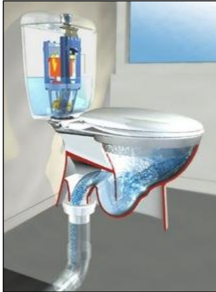
Appendix 3- Western Toilet
