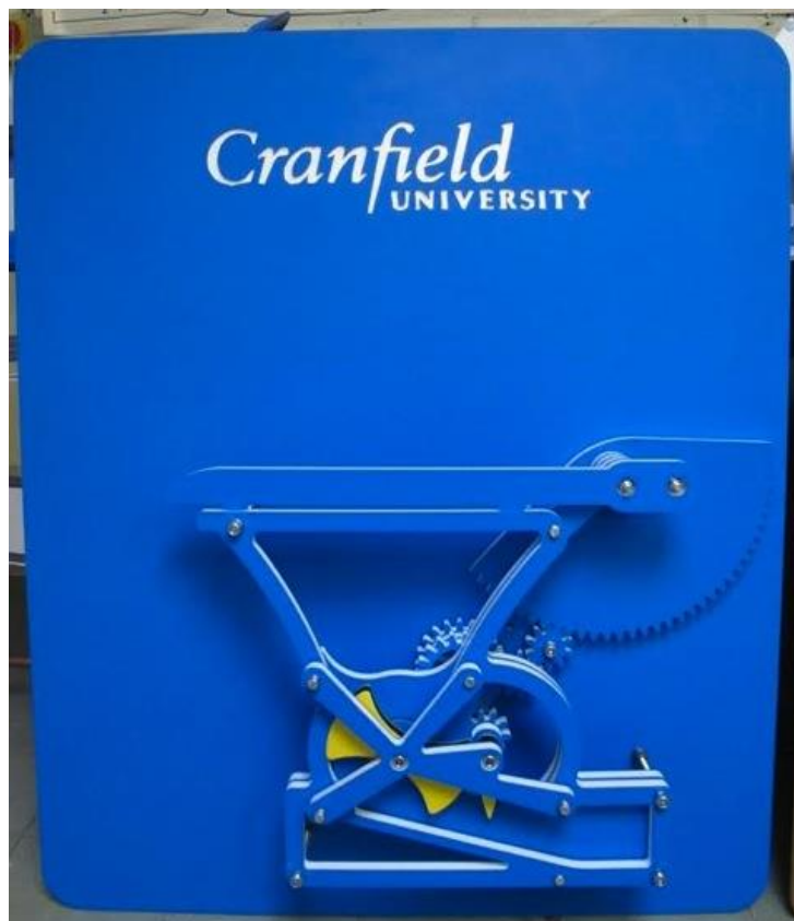
Figure 37 - Mechanism prototype rotating cup and secondary swipe all driven by the closing of the toilet lid
