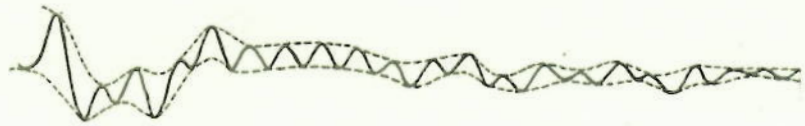
FIG. 10. A STICK JERK WITH THE ENVELOPE OF THE TRACE FROM TRANSDUCER 2 DRAWN IN FREEHAND
