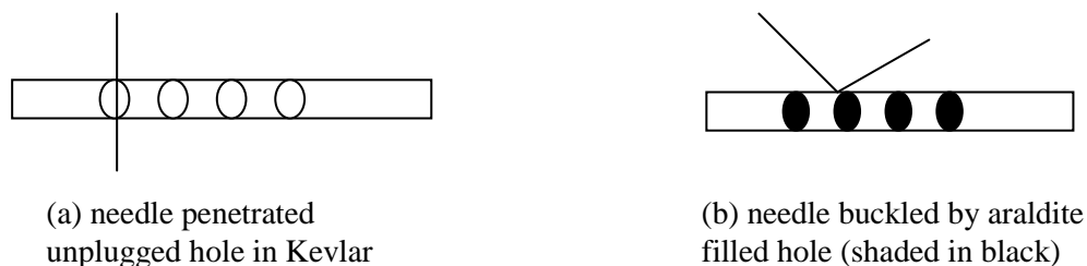
Figure 9. (a) Non-treated and (b) treated Kevlar
