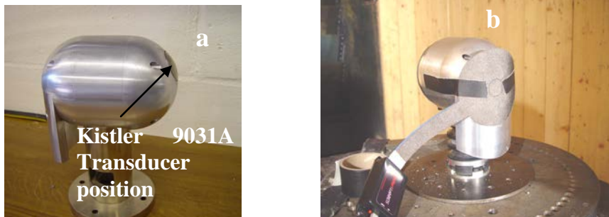
Figure 3. (a) Aluminium head form (on stand) showing position of Kistler® transducer b) Sensor attached to Aluminium head form and Hybrid 3 neck
