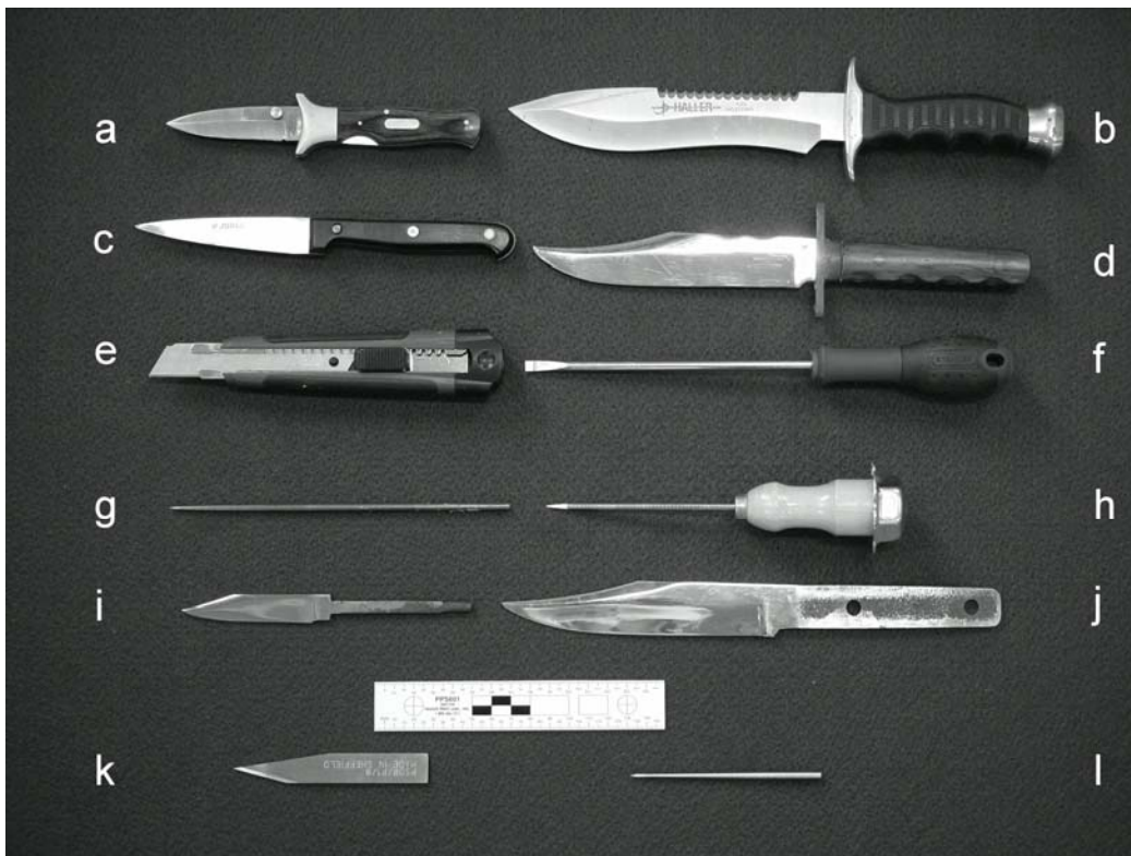
Figure 5. Typical edged weapons a) Lock knife, b) ‘Survival’ knife, c) Kitchen knife, d) ‘Bowie’ knife, e) Craft knife, f) Screwdriver, g) HP White spike (H.P. White 1988), h) American ice pick, i) PSDB N°1 test knife (Parker 1993), j) PSDB N°5 test knife (Parker 1993), k) HOSDB P1/B test blade (Croft & Longhurst 2007b), l) HOSDB Spike (Croft & Longhurst 2007b).
