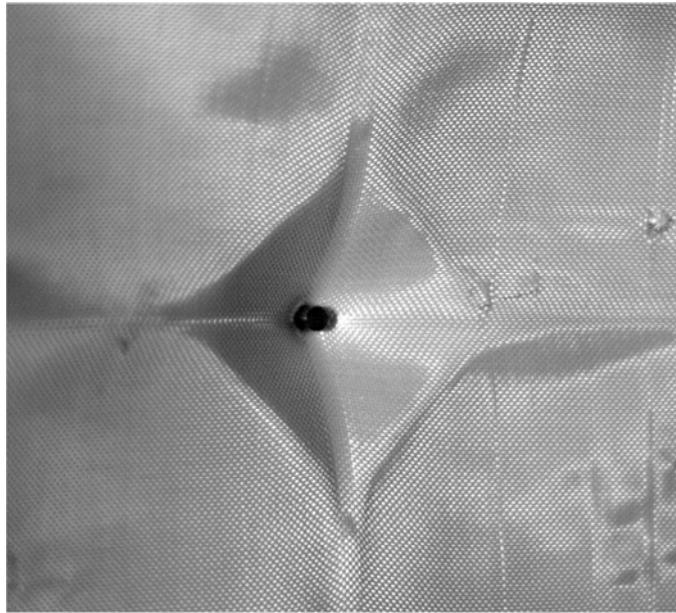
Figure 4. The pyramidal deformation of an aramid fabric during ballistic impact of a 1.1g fragment simulating projectile.
