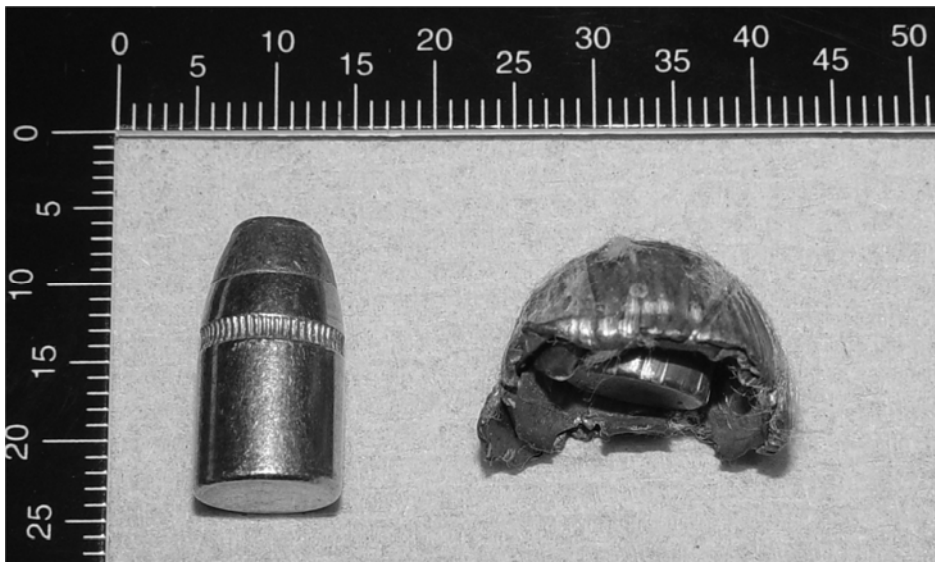
Figure 2. A .357” Magnum soft point projectile before firing (left), and deformed after impact with a textile armour (right).
