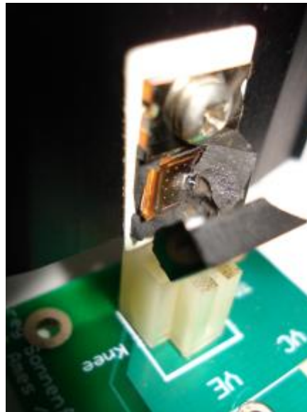
Figure 4-3 IGBT faults analysis experiment [32]
