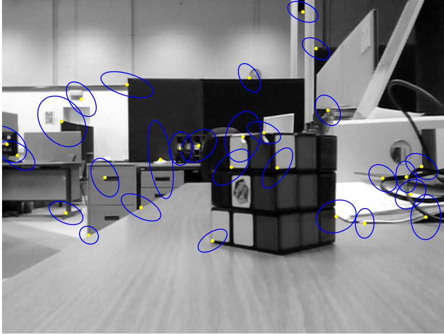
Figure 4.10: Harris features with location covariances visualised as error ellipses. The ellipses are centralised over each detected feature (yellow).
