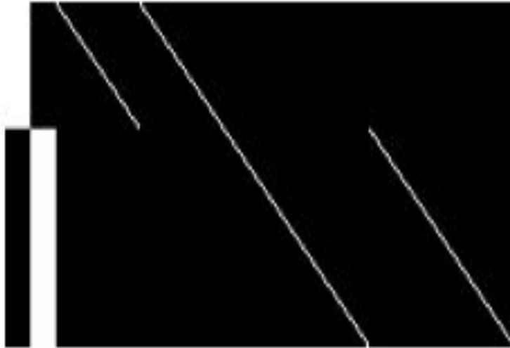
Figure 4.38: Sparse form of the J for two \mathcal{H} s and image feature points. The black spaces indicate zeros and the white lines indicate derivatives.
