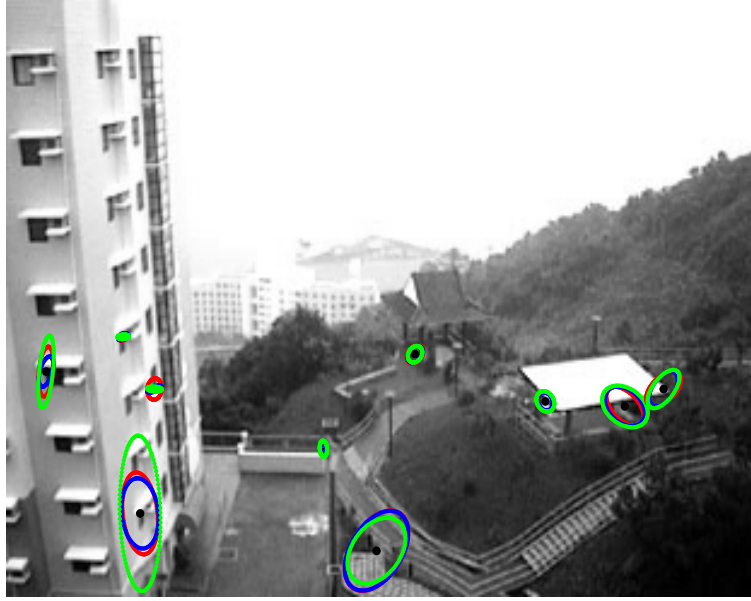
Figure 4.12: Image feature with error bounds given as ellipsoids. The three different covariances from the RGB channels are visible. Covariances from each respected channel is coloured according to its respective channel.
