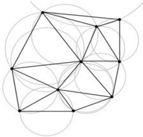
Figure 5.28: Delaunay triangulation with no points in the circum-circle given by grey lines.
