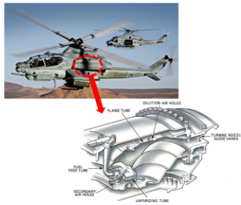
Figure 1: An annular combustor with a vaporiser and its location in Bell AH-1Z helicopter. (Source: Bell Helicopter Textron Inc. and Rolls-Royce Plc.)
