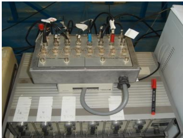
Figure 6-9: Data acquisition system (channels box)
