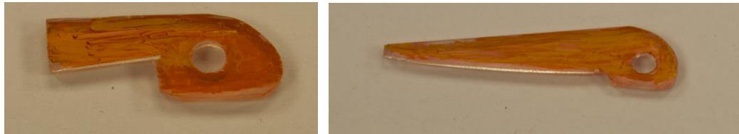
Figure 6.4 Joints of rib to wing spar
