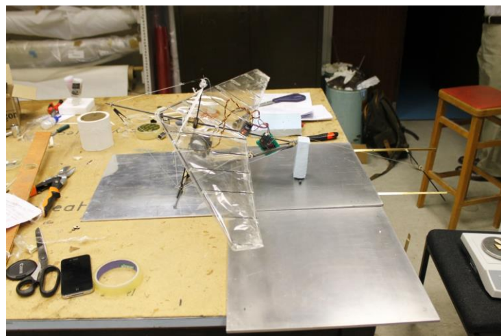
Figure 6.11 Model Test Set on Table with reduced AoA
