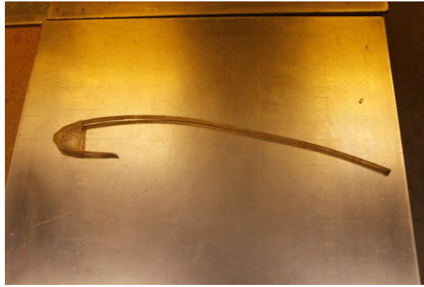
Figure 6.6 Glass fibre reinforce plastic rib
