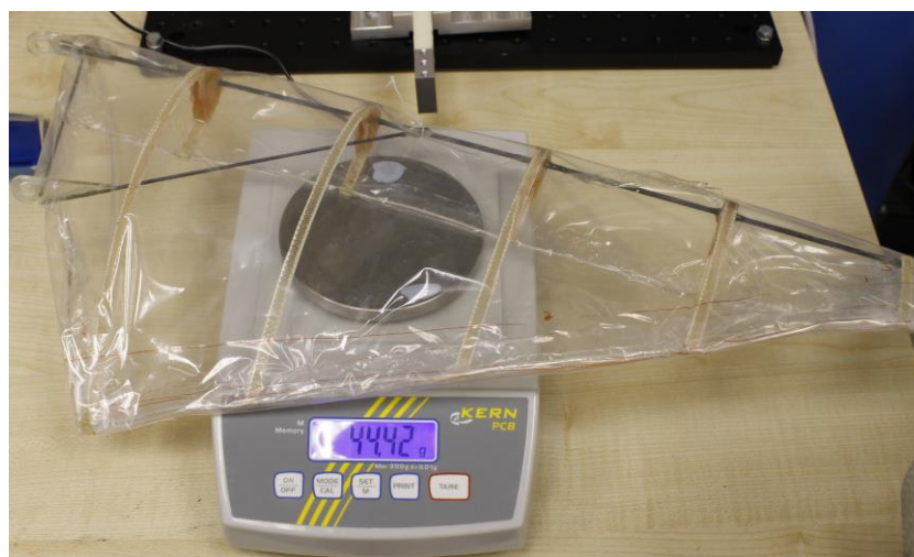
Figure 6.3 Single glass fibre reinforce plastic wing
