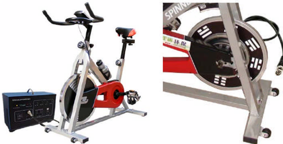
Figure 2-2 Indoor bike (left) with hub motor (right) (1)
