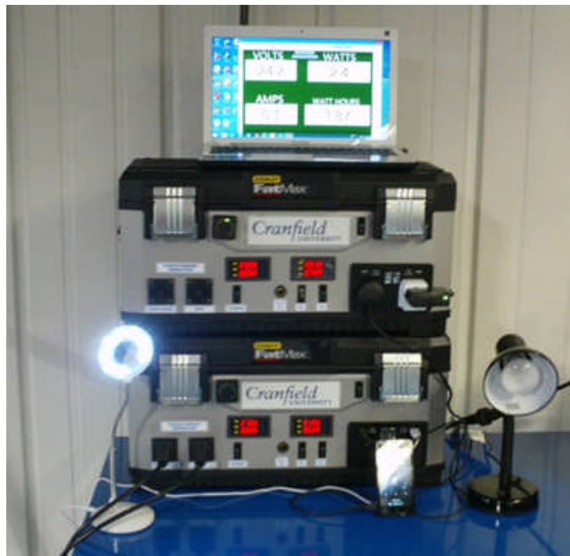
Figure 6-2 Portable power supply units
