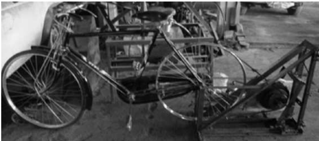
Figure 2-3 HPG with locally made low RPM generator Mechtenberg 2012
