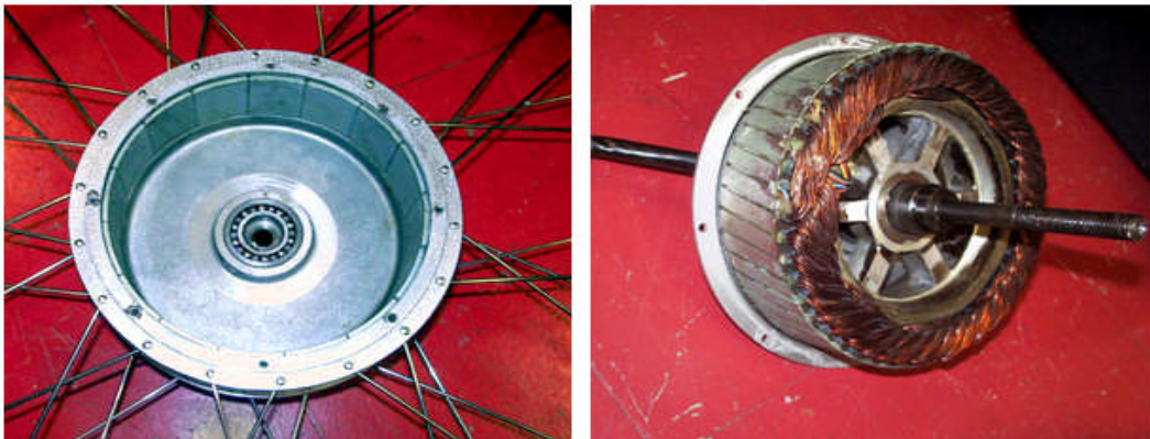
Figure 4-4 Direct-driven hub motor (5)
