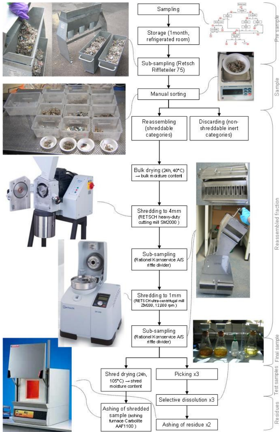
Figure 4-4 Typical sample preparation procedure followed in this thesis, exemplified for the case of biogenic content measurement. Adopted from Séverin 294 , as detailed in Séverin et al. 295
