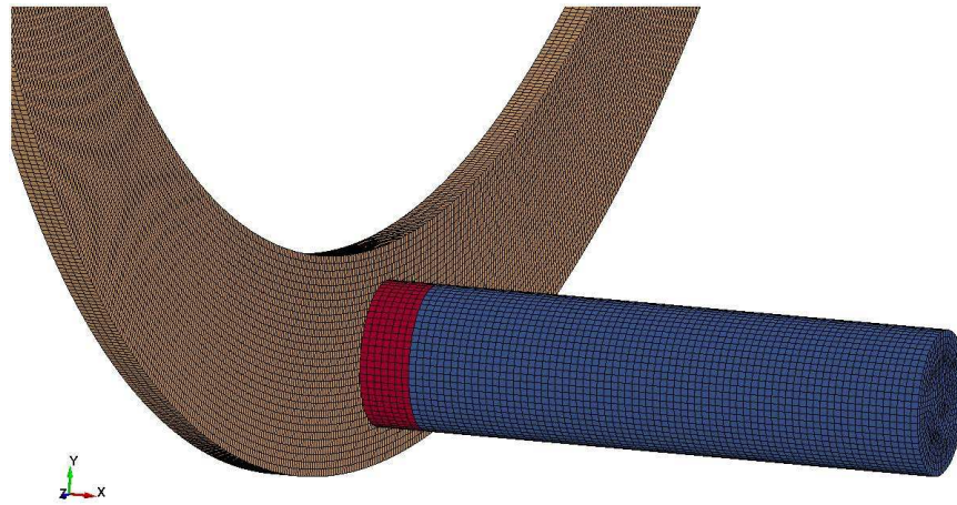
Figure 5.3: Pin-on-disc geometric model
