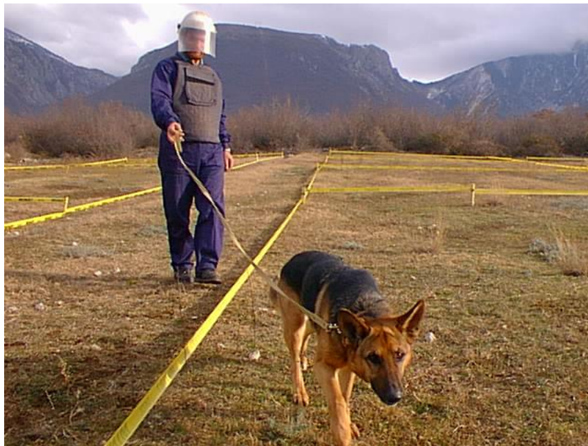
Figure 2.15: Deminer in Bosnia using a dog to survey the edge of a minefield while standing in a cleared lane (Trevelyan, 2000a)
