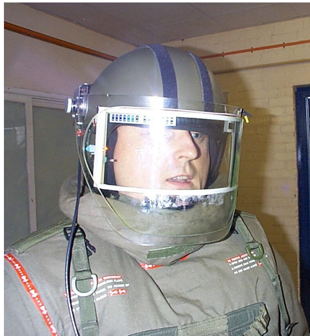
Figure 8.3: Visor demister mounted on a Mk 4 EOD Suit helmet (picture courtesy of DLO DC R&PS)
