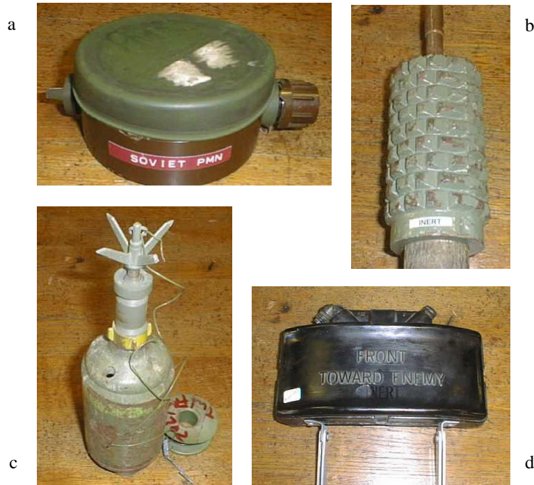
Figures 2.12a, b, c & d: AP landmines: (a) Russian PMN (blast), (b) Russian POMZ-2 (fragmentation), (c) Yugoslavian PROM-1 (bounding fragmentation), and (d) US M18A1 'Claymore' (directional fragmentation)
