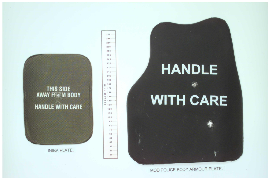
Figure 2.7: UK ceramic-faced inserts showing the (left) INIBA plate and (right) MOD Police body armour plate (picture courtesy of DLO DC R&PS)
