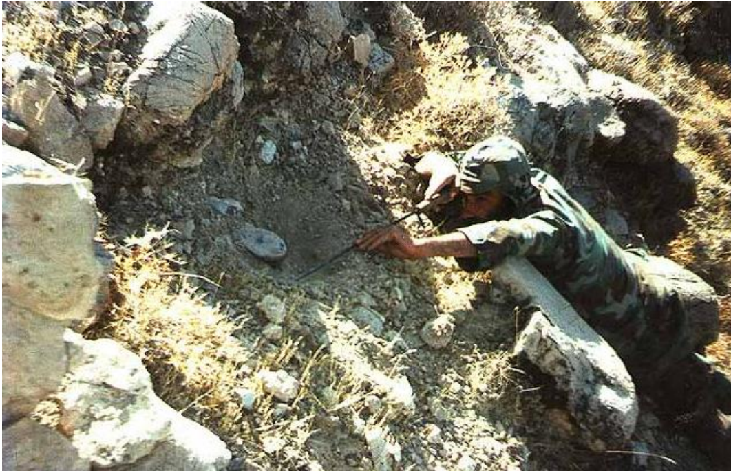
Figure 2.17: Deminer prodding around an AP blast mine in mountainous terrain in Afghanistan (Trevelyan, 2000a)
