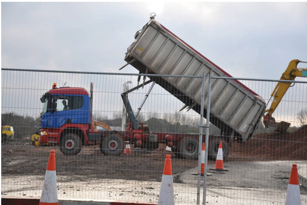
Figure 35 – Tipper body with lateral sheeting system unloading aggregate.
