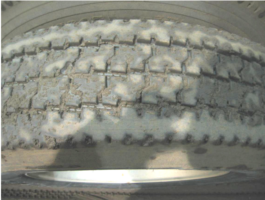
Figure 30 – Typical tyre condition after 10 passes.
