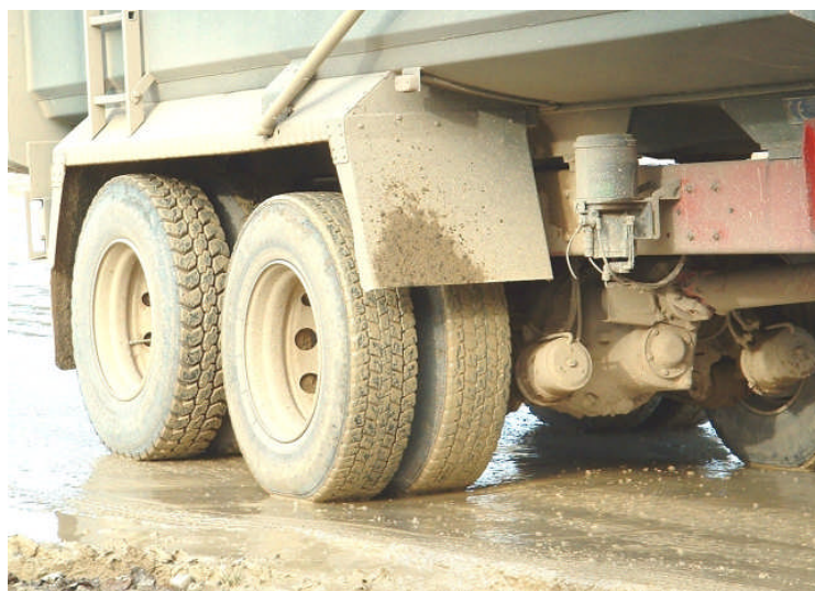
Figure 8 tyre and chassis contamination resulting from driving on unsurfaced roads within a quarry
