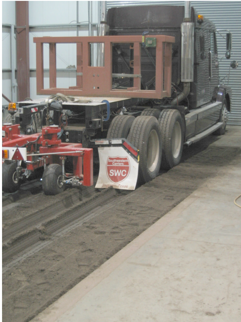
Figure 28 - 6x4 Tractor Unit used for the soil adhesion experiment within the Cranfield University Soil Dynamics Laboratory
