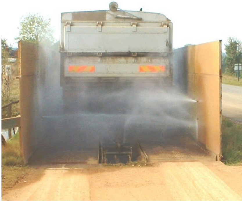
Figure 11 Automatic drive through wheel and chassis wash system
