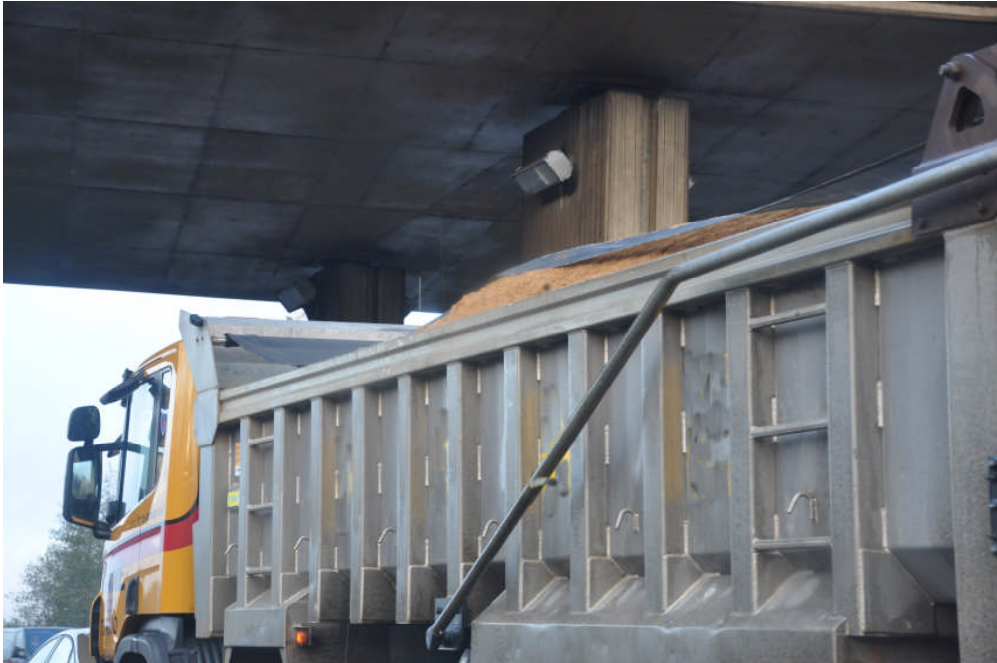
Figure 38 – Longitudinal sheet covering aggregate on an 8x4 construction truck.
