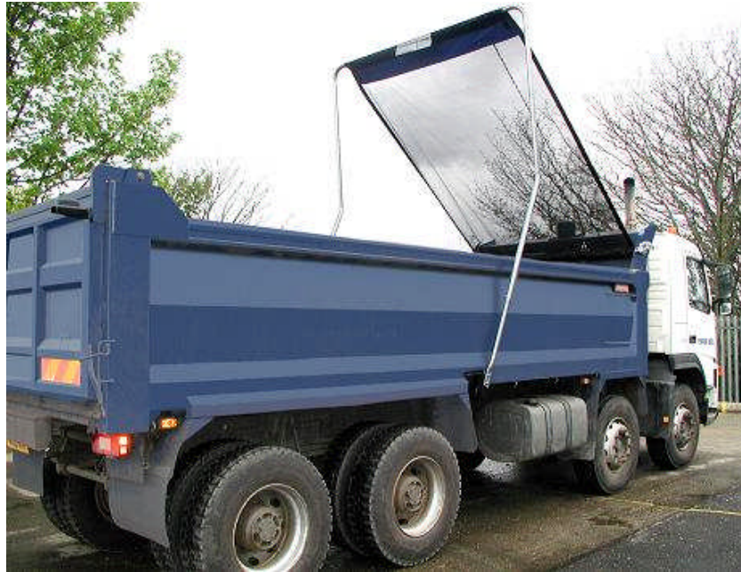
Figure 36 – Longitudinal sheet system
