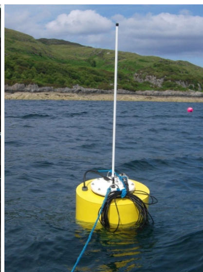
Figure 14: VRAP buoy before hydrophone cable was brought to the sea bed.
