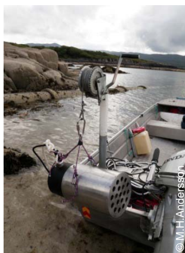
Figure 12: Winch to lower the loudspeaker from the boat.
