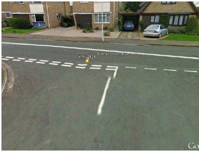
Figure 17a & b Example burst locations proximal to a road junction and subject to potential vehicle loading from waiting traffic.(Northampton, Google Street View)
