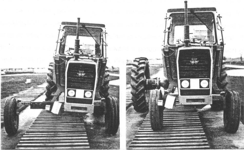
Figure 6 Track method used to excite tractor with a rear wheel input (left) and a front wheel input (right)
