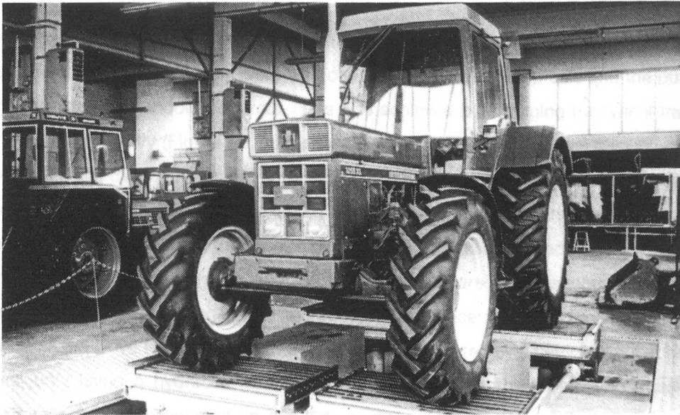
Figure 5 Four ram hydraulic test stand
