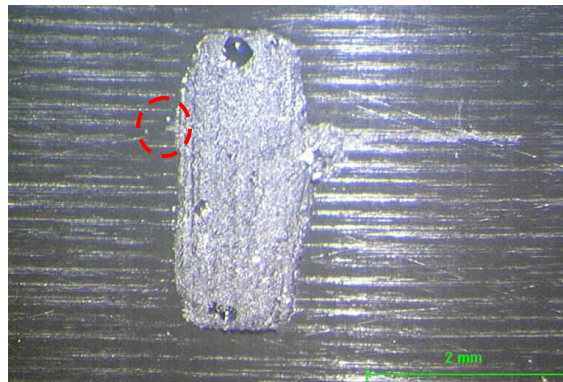
Figure 7-22: Larger scale fatigue specimen 2 - Fatigue crack initiating after 292700 cycles
