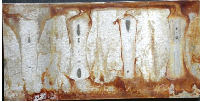
Figure 7-9: Crevice corrosion due to cylindrical crevice formers on a flat panel
