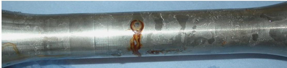
Figure 7-12: Larger scale fatigue specimen 1 after being removed from the salt spray cabinet
