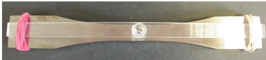
Figure 3-21: Crevice former attached to a tension test fatigue specimen
