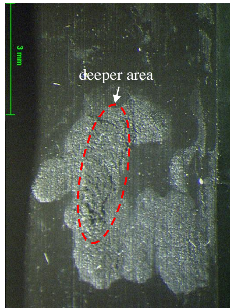
Figure 5-28: Replica of the crevice corrosion damage in specimen 10
