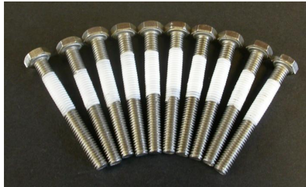
Figure 3-8: Stainless steel bolts wrapped with PTFE tape to avoid galvanic corrosion
