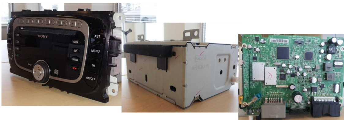
Figure 6.1 Audio head unit example: front view, rear view, and electronic main board (left to right)
