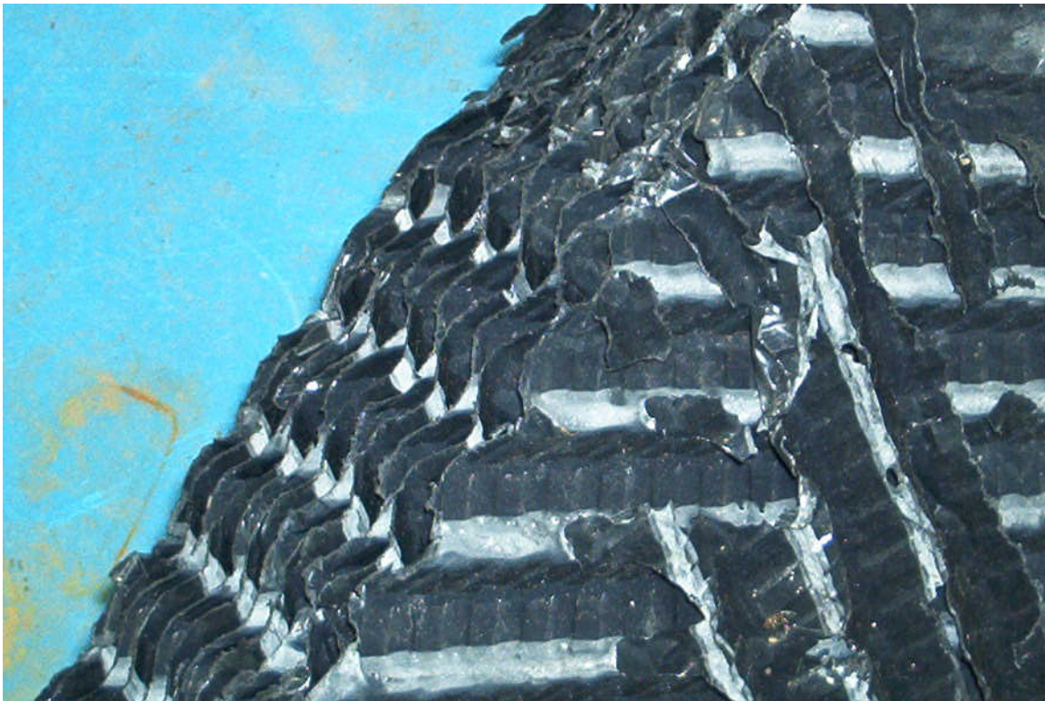
Figure 5.7 BIOdek media showing two sides and the structure with diagonal corrugation in opposite directions.
