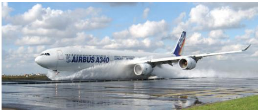
Fig. 1.6 Spray ingestion from landing gear constraint: example of an engine injection test. (Rivoire, 2007).
