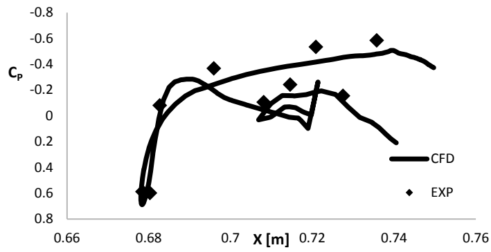
Fig. 6.19 Slat numerical and experimental slat C_p at \eta = 0.50 , \alpha = 6^\circ .
