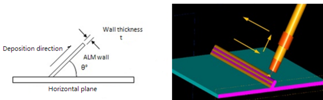
Figure 4.5: Definition of wall deposition angle \theta
