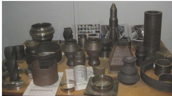
Figure 2.4: Products manufactured by WAAM
